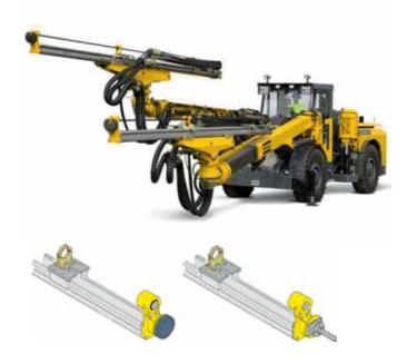
The front and middle guides are replaced to an application specific design for easy handling of the pipes.
